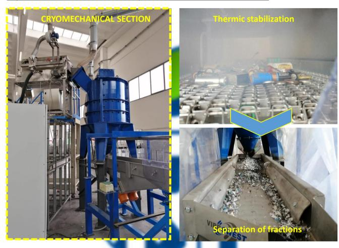
Cryomechanical treatment includes thermal stabilization with liquid nitrogen, crushing and subsequent separation of ferrous fractions, plastic residues and electrodic powder.
